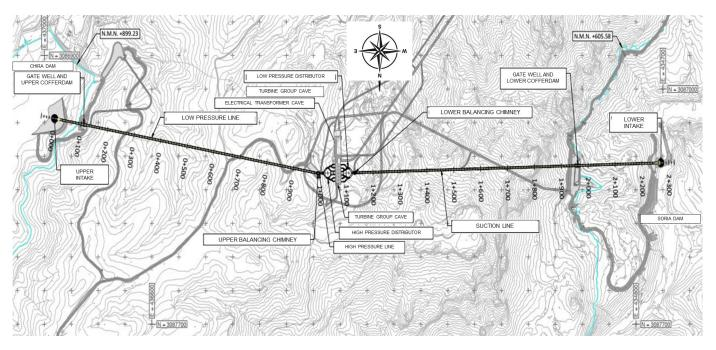
**Figure 5.** General plan of the Hydraulic Circuit, with the Chira reservoir on the right and the Soria reservoir on the left in this image (image oriented south instead of north).
