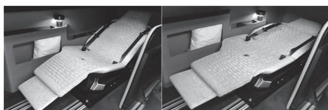
Fig. 2. Prototype seat and environment in the reclined (left) and flat (right) seat positions.
