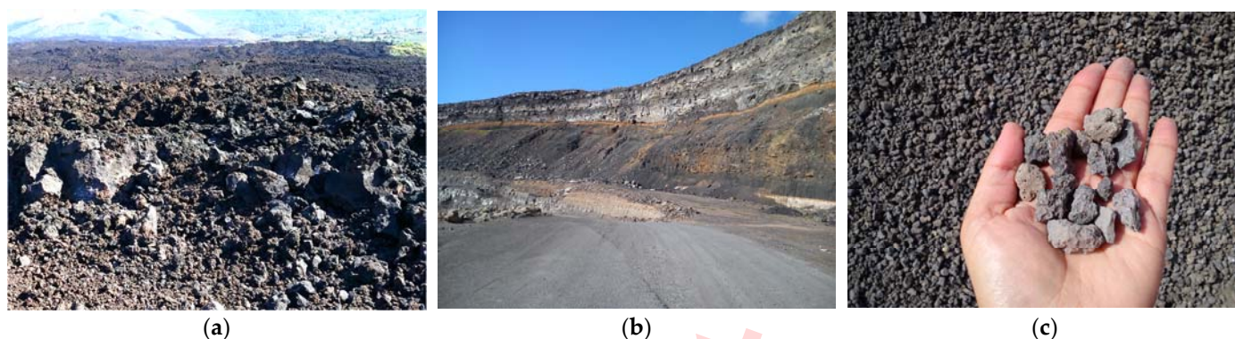
Figure 1. Vesicular volcanic aggregates: (a) rock structure of a lava flow; (b) typical heterogeneity, variability, and discontinuous special distribution of volcanic rocks in a quarry; (c) detail of the fraction 10–20 mm.
