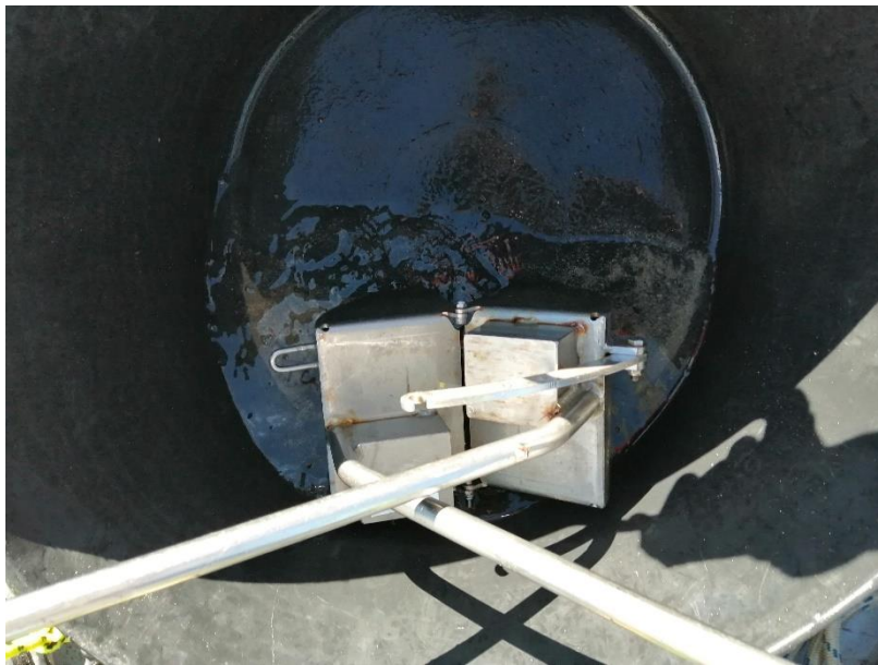
Fig S1. Pictures of the Van Veen dredge that was used for submerged sampling collection.
