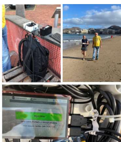
Fig 2. In situ gamma spectrometry measurement process with KATERINA II detector.
