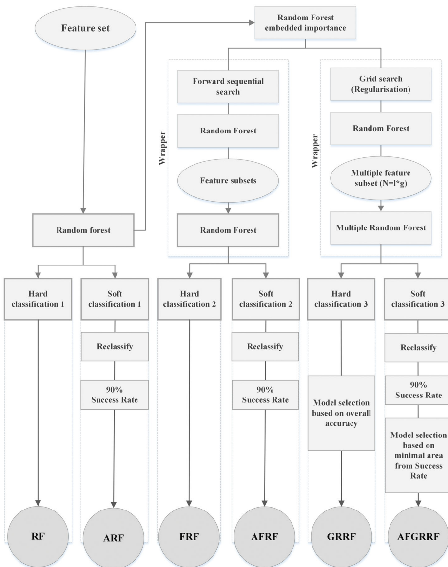
Figure 3. Flowchart with the Random Forest (RF) based methods used in this study to benchmark the proposed Area and Feature Guided Regularised Random Forest (AFGRRF). The performance of our proposed method was compared to (i) standard RF; (ii) Area Random Forest (ARF); (iii) Feature Random Forest (FRF); (iv) Area Feature Random Forest (AFRF) and (v) GRRF. The hard classification methods (RF, FRF and GRRF) produce categorical maps, considering by default an arbitrary threshold value of 0.5 in the class conditional probability. The soft classification methods (ARF, AFRF and AFGRRF), which predict a class conditional probability, were assessed in terms of the smallest affected area at a true positive rate equal or higher than 90%.
