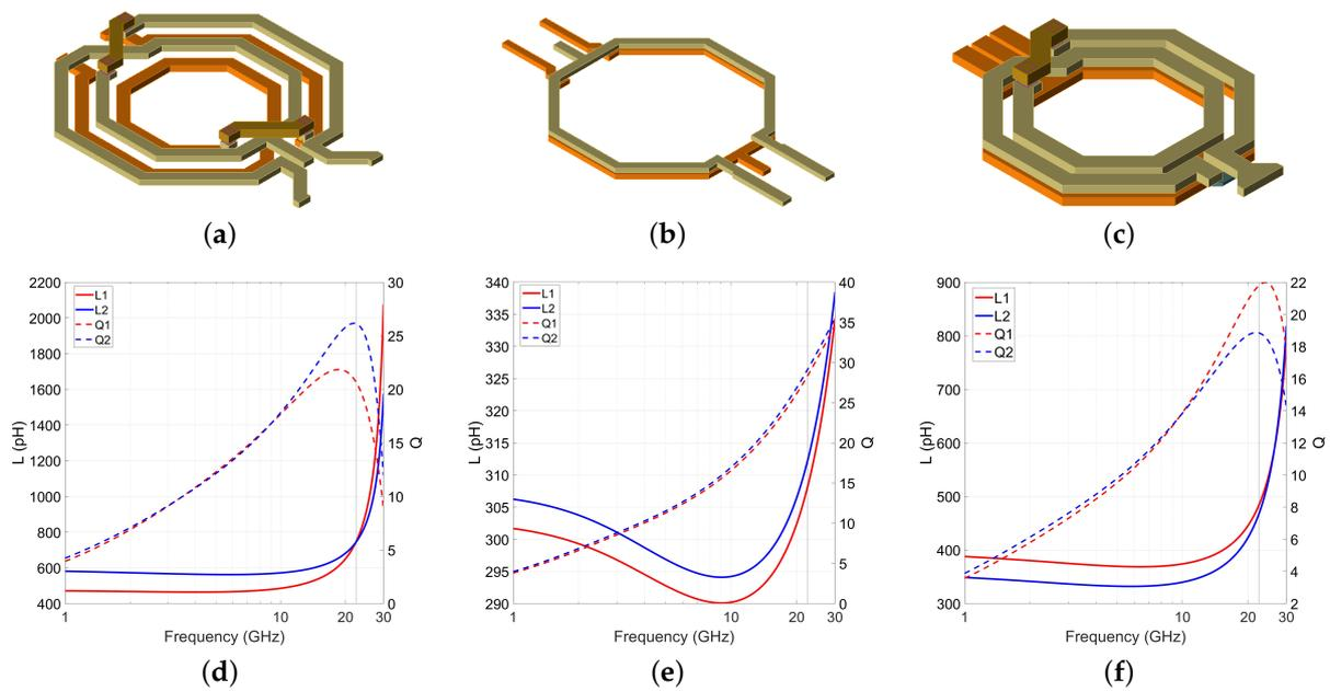
**Figure 5.** Layout of the input transformer T1 (a), the second transformer T2 (b), and the output transformer T3 (c), and inductance, and quality factor of transformers T1 (d), T2 (e), and T3 (f).
