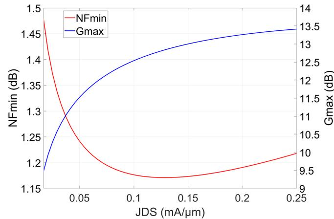
**Figure 2.** Simulated  $NF_{min}$  and  $G_{max}$  as a function of the device current density  $J_{DS}$  at 22.5 GHz.
