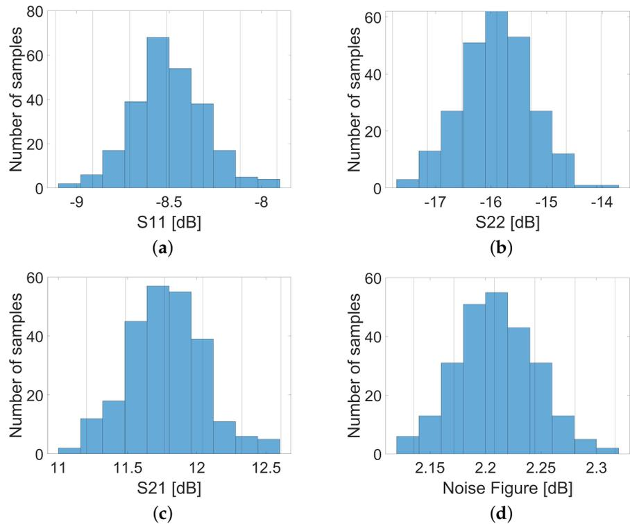
Figure 8. Monte Carlo analysis results of the IRL (a), ORL (b), gain (c), and  $NF$  (d) of the proposed LNA at 22 GHz.
