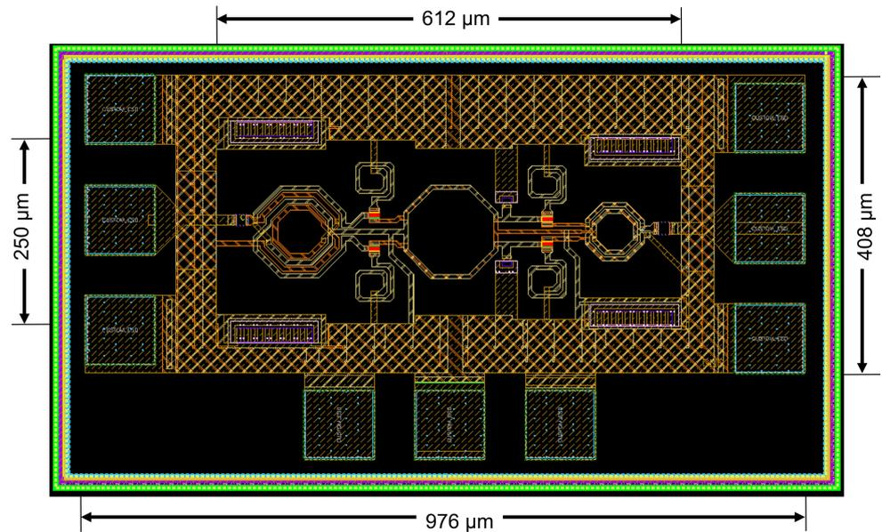
Figure 7. Layout of the proposed LNA.
