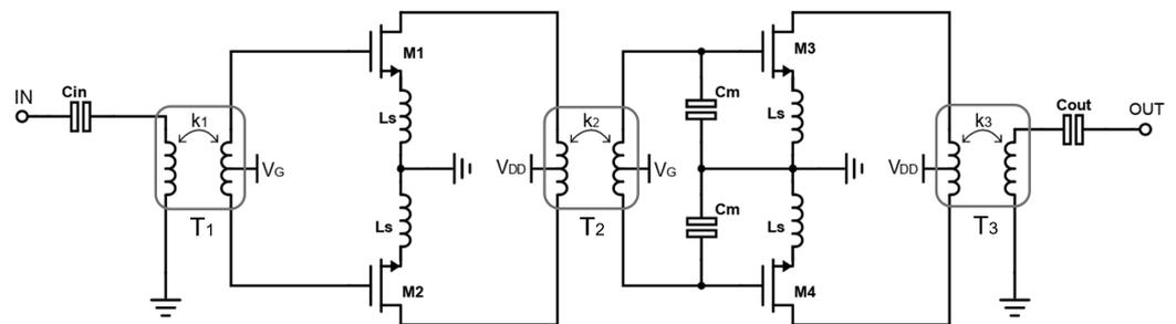
**Figure 1.** Schematic of the proposed fully differential 2-stage LNA with transformer-based interstage matching networks.
