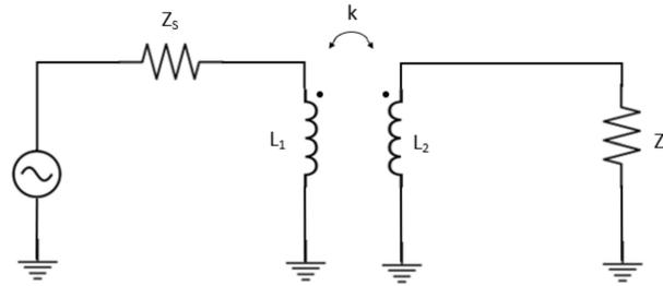
**Figure 4.** Equivalent circuit of a transformer-based impedance matching network.
