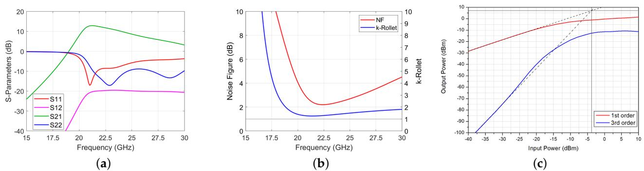
**Figure 6.** Simulated S-parameters (a) and  $NF$  and Rollet stability factor (b), and input and output third-order intercept of the developed LNA (c).
