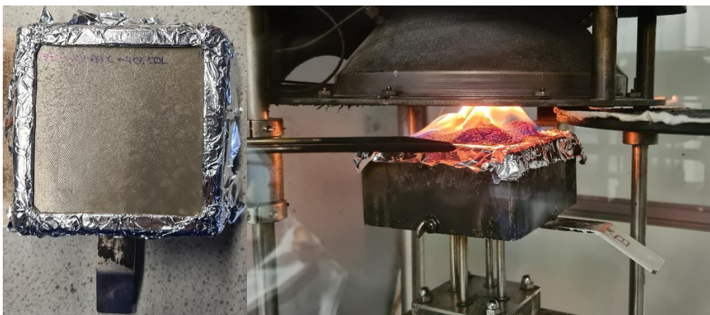
FIGURE 20: CONE CALORIMETER SAMPLES WITH RETAINING FRAME
