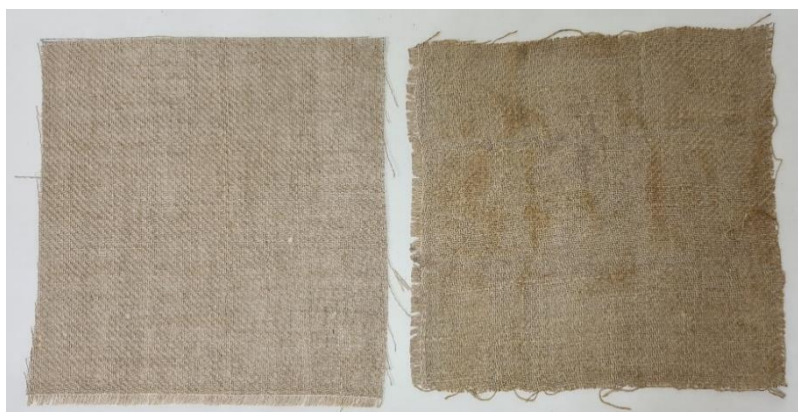
FIGURE 8: LINEN FABRIC BEFORE AND AFTER TREATMENT WITH BPS
