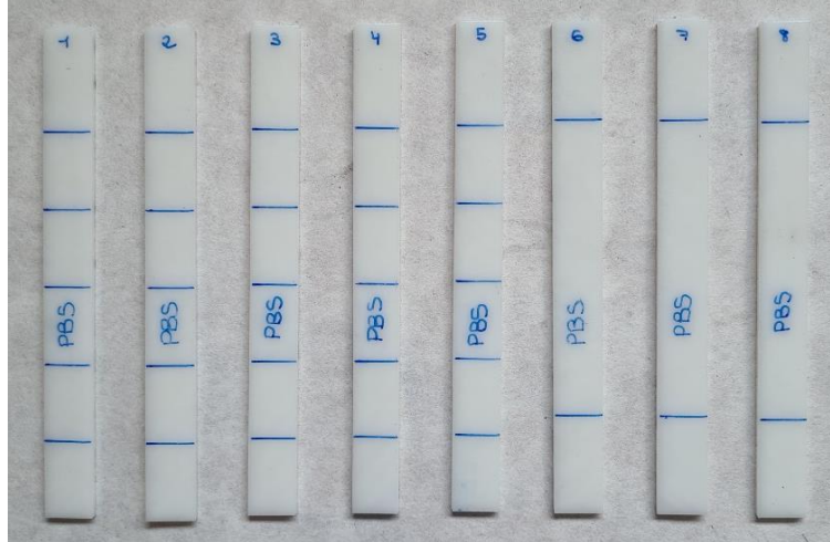
FIGURE 19: SAMPLES PREPARED FOR UL94 TESTS
