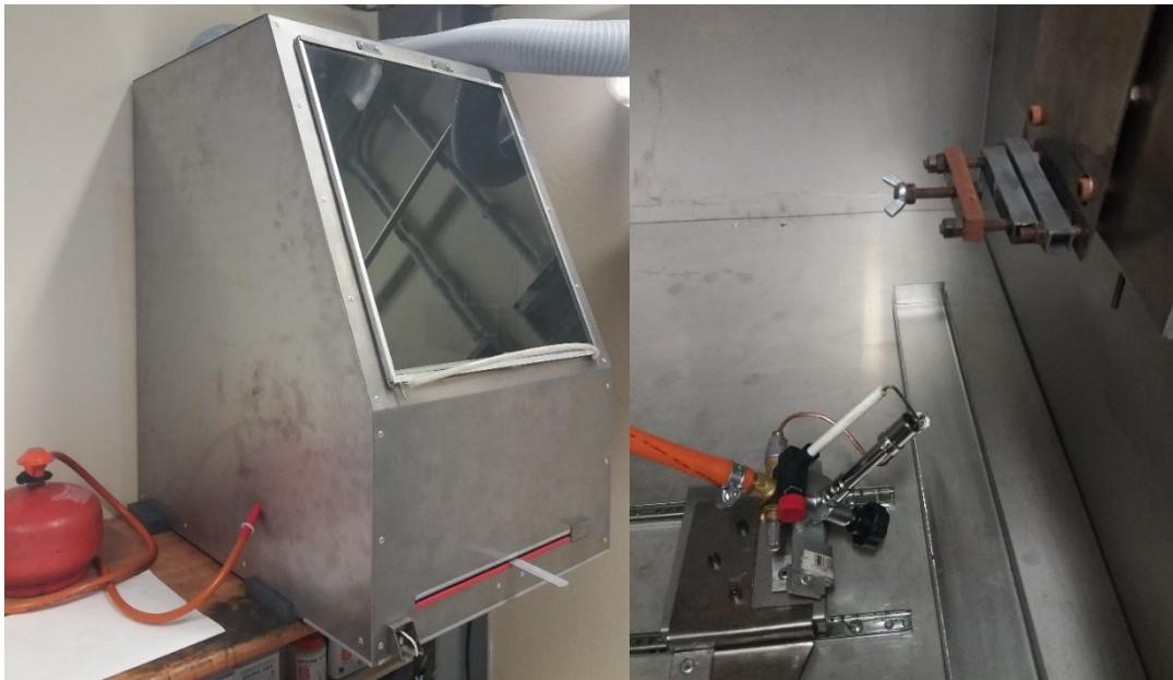
FIGURE 18: FIRE TEST LAB-MADE EQUIPMENT
