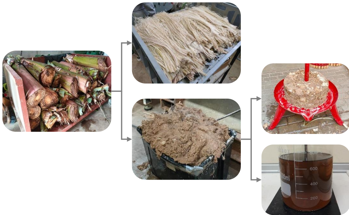
FIGURE 1: BANANA PSEUDOSTEM SAP EXTRACTION
