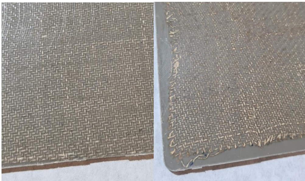
FIGURE 2: COMPARISON OF COMPOSITES WITH UNTREATED (LEFT) AND TREATED (RIGHT) LINEN FABRIC
