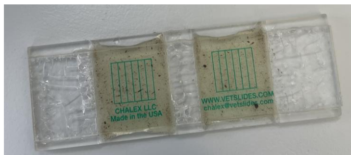
Figure 9. Compartment of the count cell. Each compartment has a surface area of 10 x 10 mm, with a space between object-glass and coverslip of 1.5 mm (Thienpont et al. , 1979).
