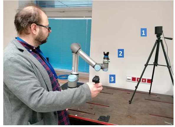
Fig. 6. UR5 teaching by man-operator using Mimicking Kit tracker in laboratory environments: 1 is the infra-red Transmitter sensor, 2 is the Receiver antenna, 3 is MK joystick hold in operator's hand.
