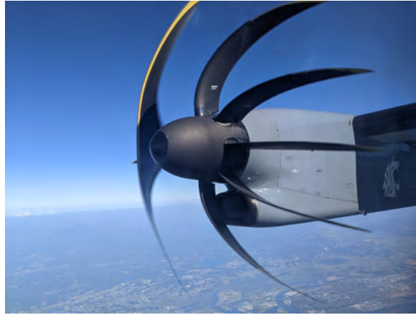
Figure 3.2: A de Havilland Canada Dash 8 propeller, with severe RS distortion from a Pixel 3 camera by Dicklyon (Wikipedia).
