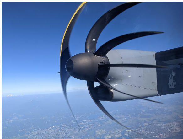
Figure 3.2: A de Havilland Canada Dash 8 propeller, with severe RS distortion from a Pixel 3 camera by Dicklyon (Wikipedia).
