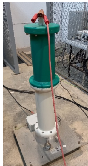
Figure 8. Reference capacitor, Haefely Test AG, rated capacitance 100 pF, rated voltage 100 kV, dissipation factor 1 \times 10^{-5} .
