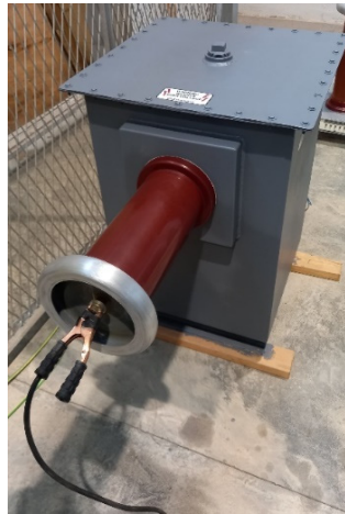
Figure 9. HV test transformer model HHT7-10T-220, Hipotronics-Hubbell, rated input 230 V AC, 10 KVA, rated output 100 KVA, 100 mA, freq. 50 Hz.
