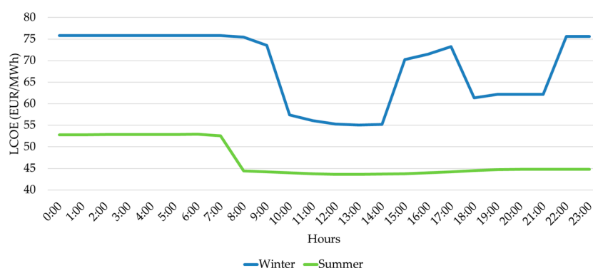
Figure 9. LCOE of the diversified renewable generation system for a typical winter and summer day.
