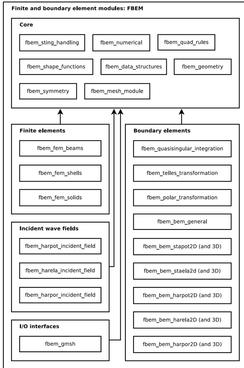
Fig. 3. FBEM library of modules corresponding to the computational layer of MultiFEBE.
