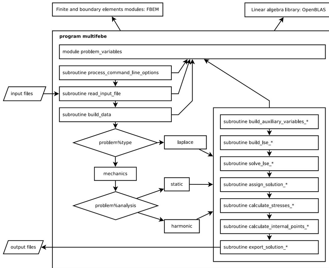
Fig. 2. Overview of the general architecture of the MultiFEBE code. Application layer.
