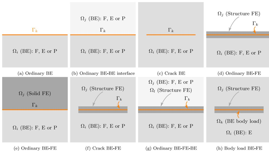
**Fig. 1.** Type of Boundary Element (BE) and Finite Element (FE) situations, including coupling between them. BE region material models are denoted as: inviscid fluid (F), elastic solid (E), poroelastic medium (P).
