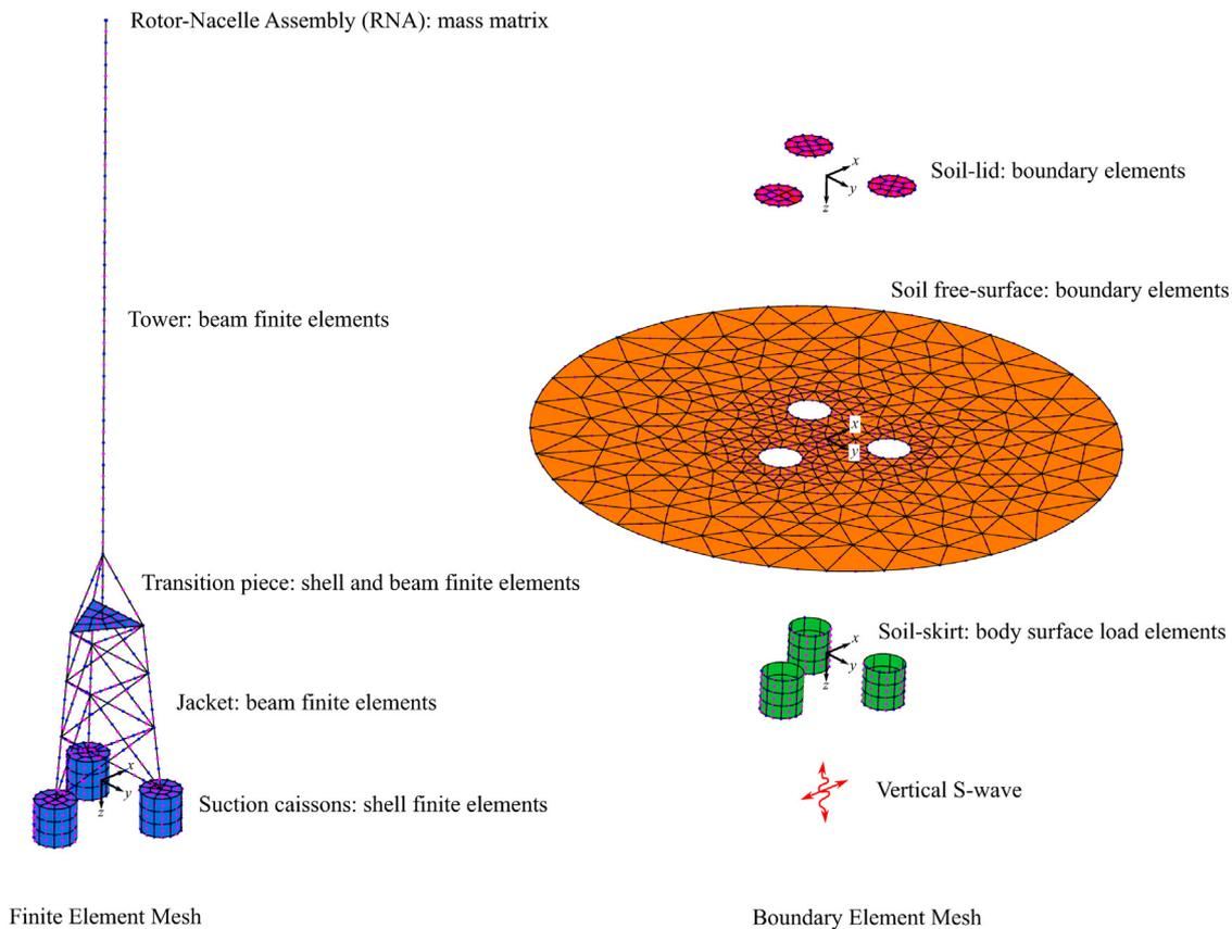
**Fig. 4.** Exploded view of a coupled model of finite elements and boundary elements for the dynamic analysis of an offshore wind turbine.
