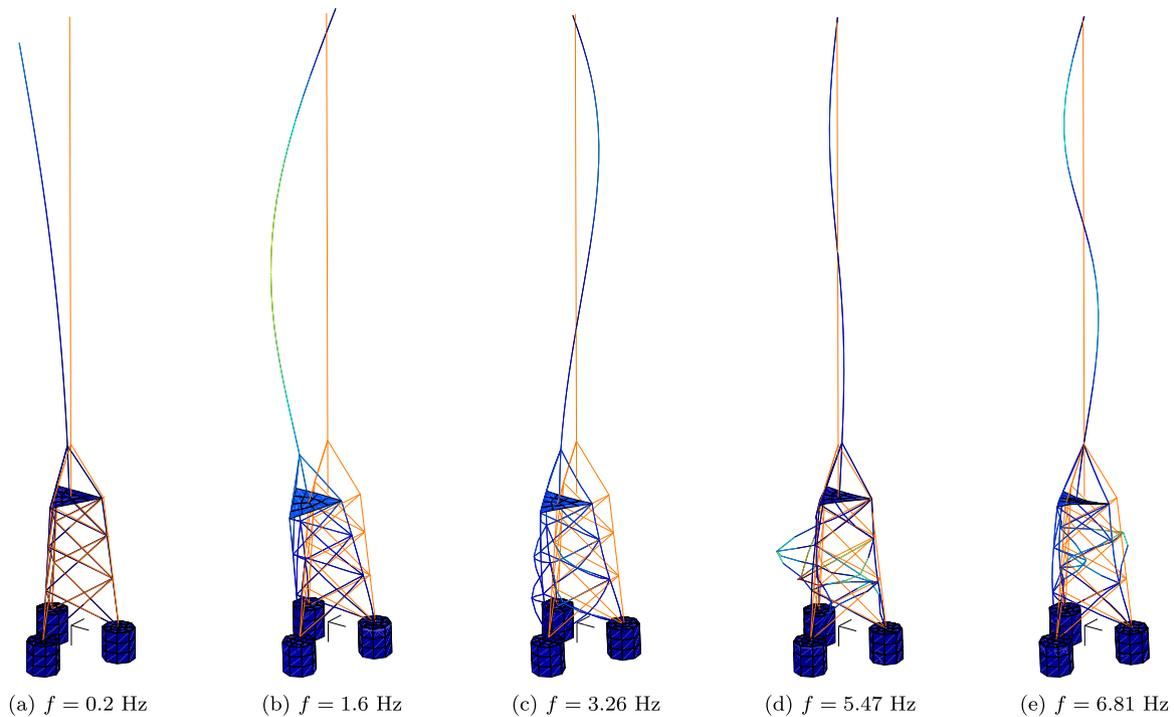
Fig. 6. Deformed shapes of the offshore wind turbine structure at different frequencies.
