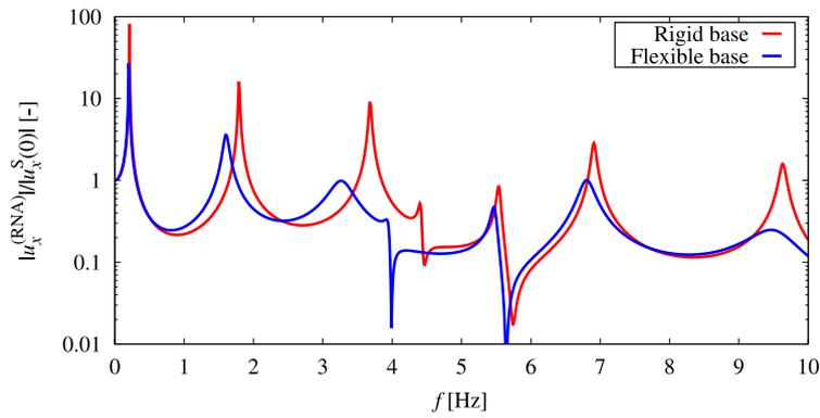
Fig. 5. Normalized horizontal displacement response at the tower top.
