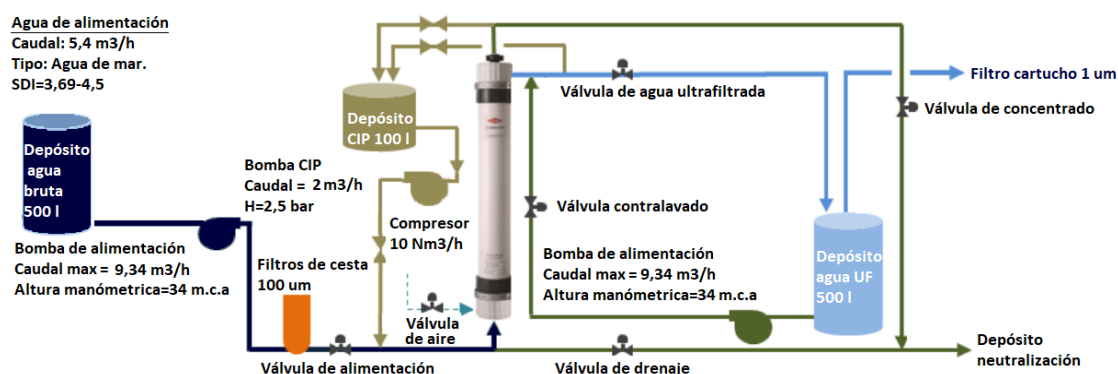
Figure 2: Process diagram of the UF pilot plant.
