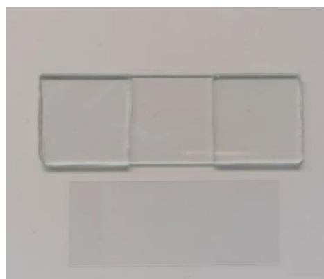
Figure 2: Home-made chamber used in the qualitative analysis of the samples.
