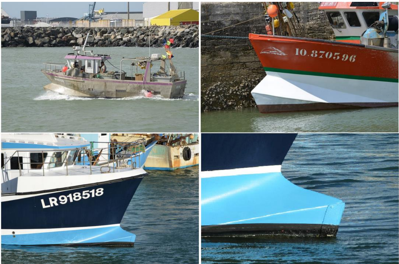
Figure 1. Examples of polyhedral bulbous bows. ( https://commons.wikimedia.org/wiki/Category:Polyhedral_bows (accessed on 1 September 2022)).
