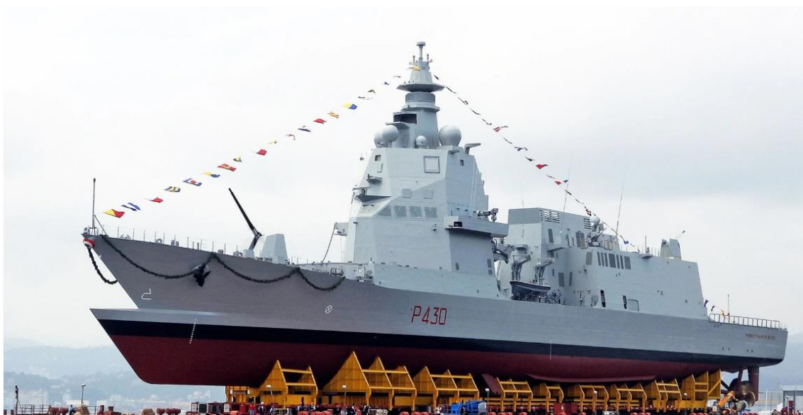
Figure 27. Paolo Thaon di Revel ship with a polyhedral bow. https://www.armadainternational.com/2019/07/italian-navy-launches-paolo-thaon-di-revel/ (accessed on 1 September 2022).
