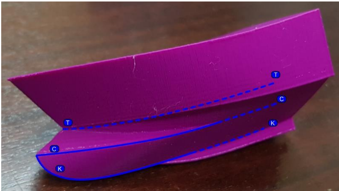
Figure 4. Example of curves; T curve inside the hull.
