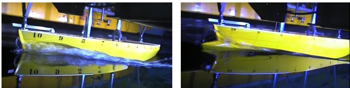
Figure 19. FAO1 vs. FAO2 at 7.5 kn, Heavy condition.
