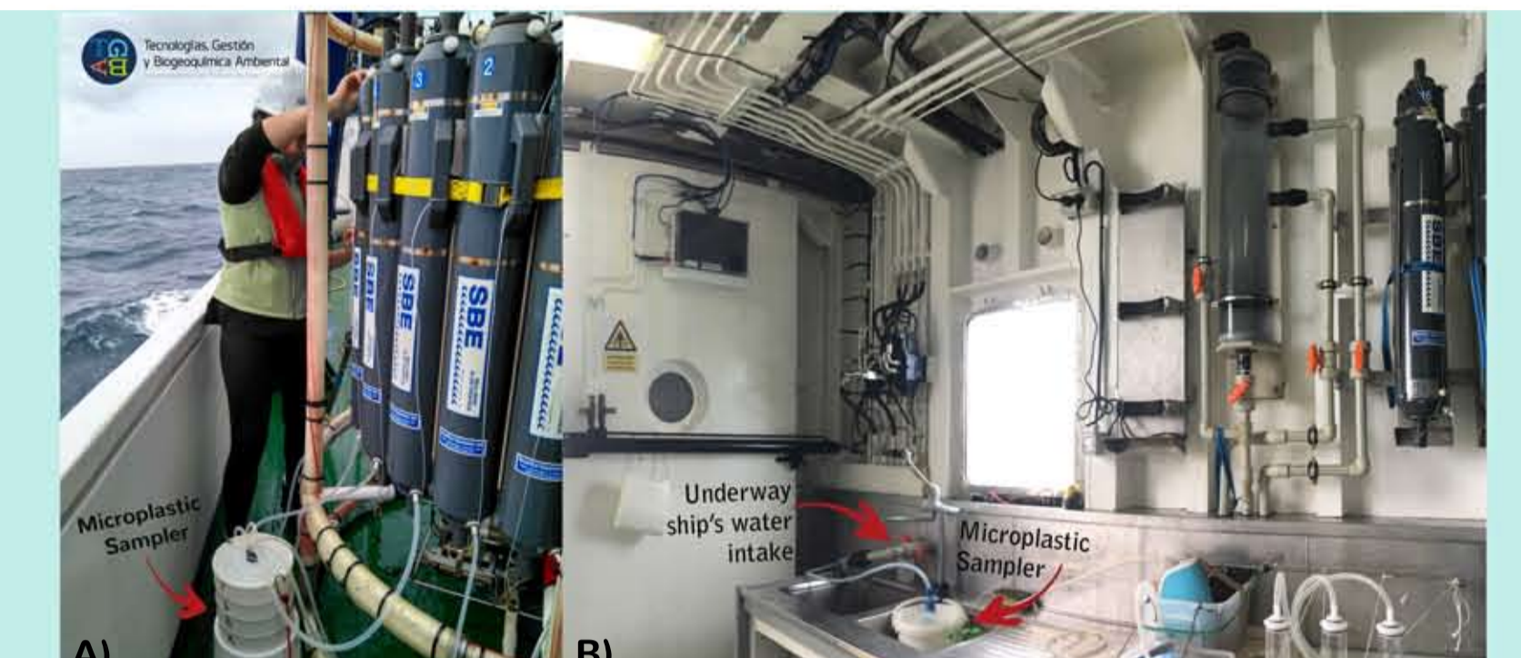
Fig. 3 Filtering procedure onboard the R/V Ángeles Alvariño: A) Water collected by the Niskin bottles from the Rosette Sampler, B) Connected to the underway seawater intake system.
