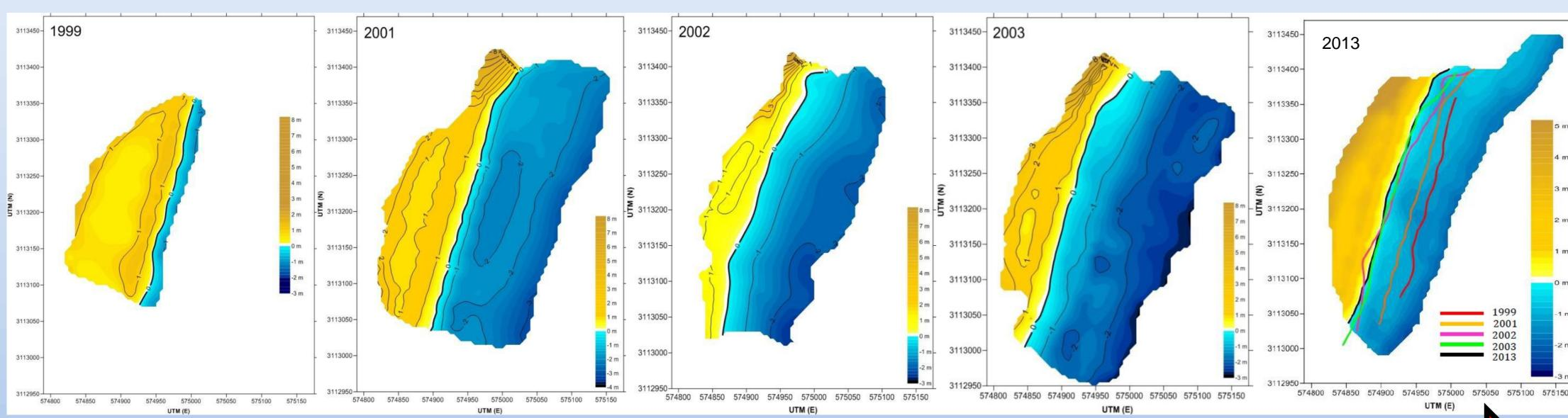
As the years progress the outside of the beach gets eroded and this has as a main consequence the retreat of the coastline an disappearance of the sand bar.
