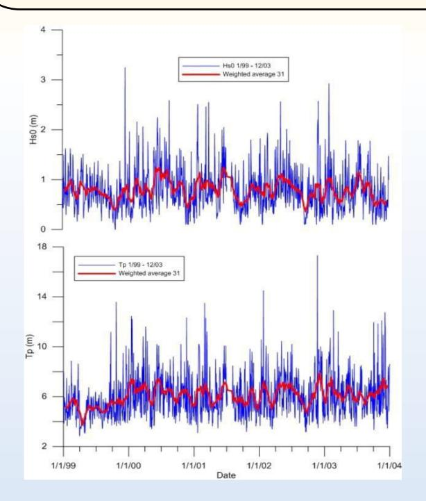
To determine the causes responsible of the measured coastal retreat climatological data were used. Wave data were provided by Puertos del Estado (<u>www.puertos.es</u>) corresponding to WANA 1024012 point, the closest to the study area. The data set included Hs, Tp and approaching wave direction, covering a 5 years period from January 1999 to December 2003, with one data every 3 hours.
