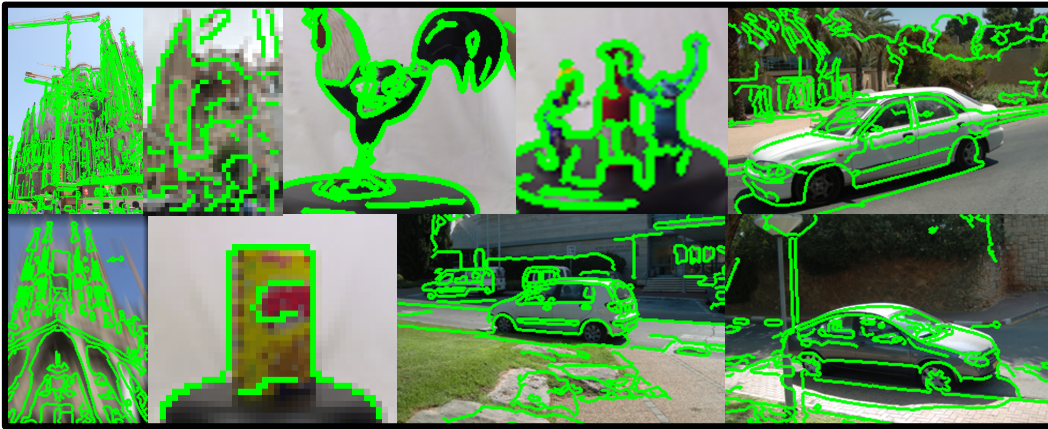
Figure 7. Pose estimation results represented as reprojected wireframes of the best matching candidate in the training data. Although our pose is better than the closest image from the training set, we do not directly project the 3D model point cloud because it would clutter the image in an unintuitive way.
