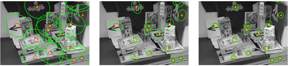
Figure 3: Limiting the number of potential candidates. Left: Search region obtained after projecting the three terms of Eq. 2 independently. Center and Right: Refinement of the search space, after establishing correspondences.
