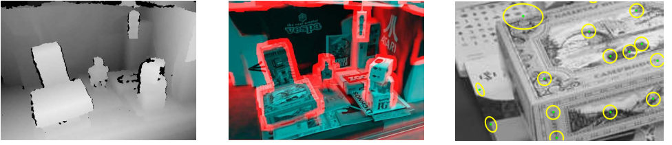
Figure 2: Uncertain 3D model. Left: 3D model acquired with a Kinect camera. Regions in which the 3D data is most uncertain are depth discontinuities. Center: We detect the uncertain regions –shown in red– computing depth covariances within local neighborhoods. Right: A 3D covariance is assigned to each 3D model point and propagated to the image plane. This is used to limit the area where to search for potential match candidates.
