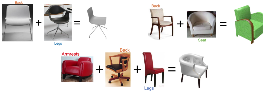
Fig. 1. Our approach takes two (or more) inputs, either RGB images or 3D models, and part labels such as “ legs ” or “ backrest ” and retrieves a shape that combines object parts or properties from all inputs, via a cross-manifold optimization technique.
