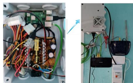
Fig. 8: Raspberry Pi, Power Supply, Access Point, Switch, Wibeec and Differential.
