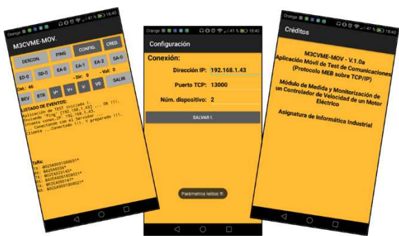
Fig. 13 - Mobile client application
