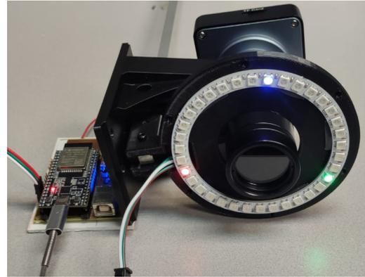
Fig. 5. Image of the lighting system during development.
