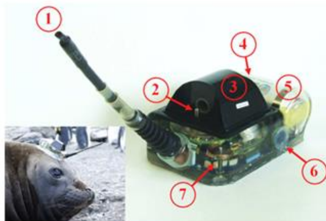
Figure 10: CTD-Satellite Relay Data Logger (CTD-SRDL) with antenna (1), temperature sensor (2), inductive cell (3), pressure sensor (4), battery (5), communication port (6) and wet-dry sensor (7) (Boehme et al. , 2009).
