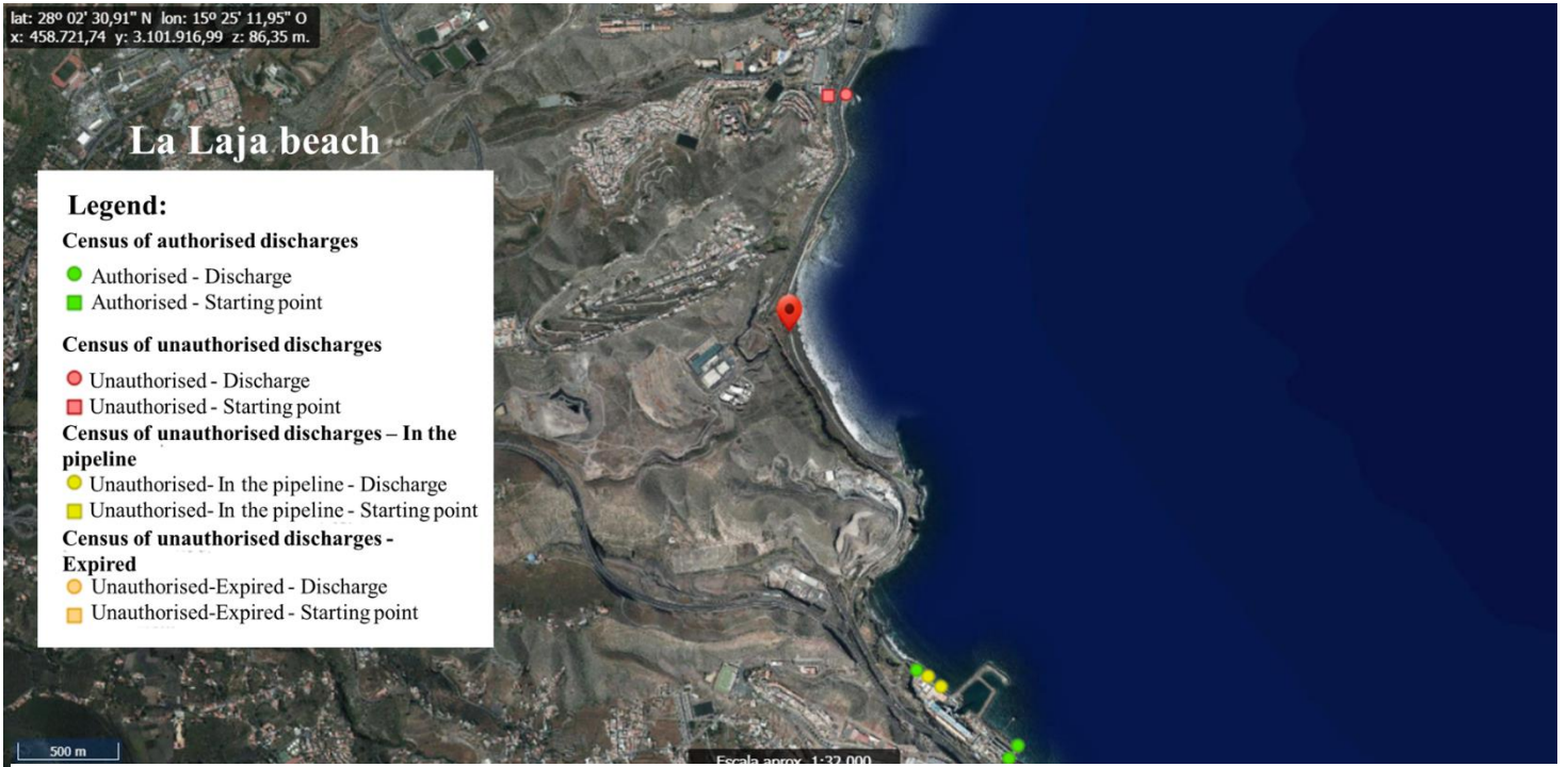
Figure 15. Wastewater discharges near La laja beach.
