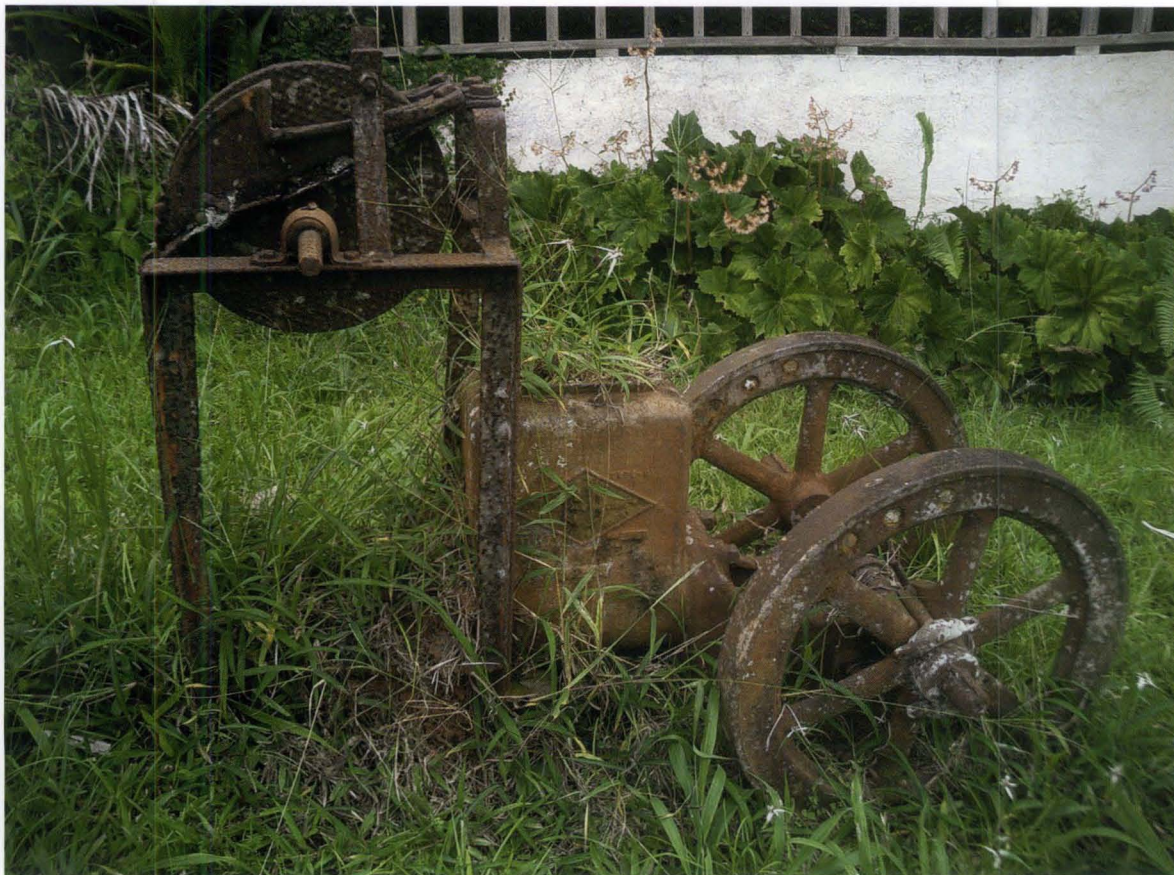
Fig. 5. Vestiges of Puerto Rico's heyday of coffee production are scattered across the landscape, such as this Emerson-Bratigham engine for removing the pulp from the coffee beans. (Photo courtesy of the author).
