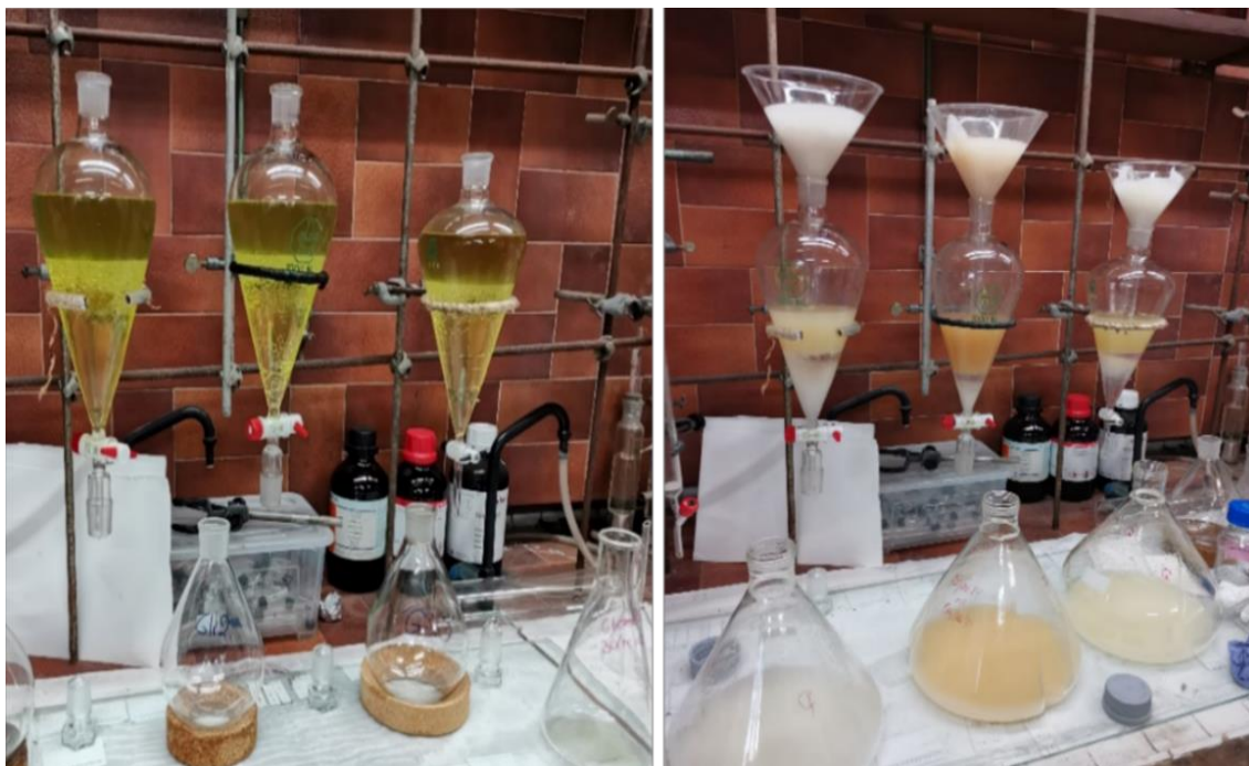
Figure 8. Photograph of the process of culture extractions (A) Enriched Symbiodinium sp. , (B) Bacterias.
