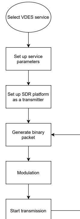
**Figure 2.** Proposed transmission flow chart
