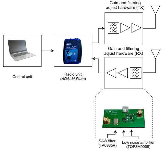
**Figure 1.** Block diagram of the prototype's architecture
