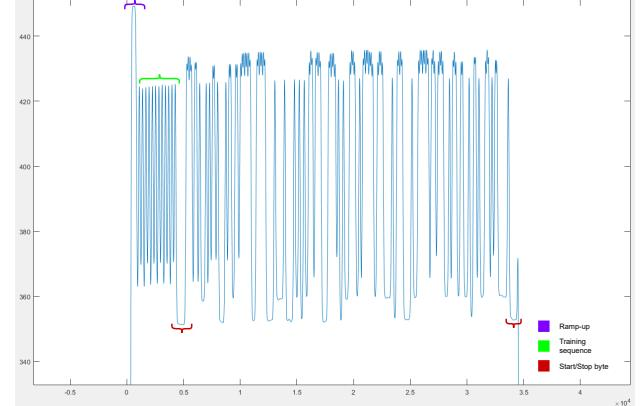
Figure 5. Analysis of an AIS signal received in time domain
