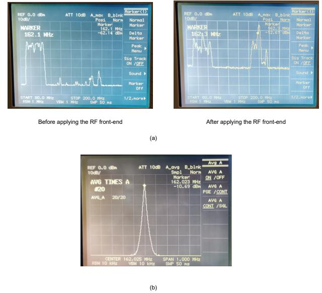
Figure 4. Spectrum without (left) and with (b) filtering and amplification hardware
