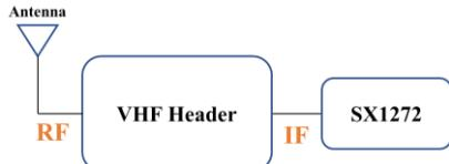
**Figure 1:** Block Diagram of the system. The VHF header transmits/receives RF to/from the antenna. VHF header also transmits/receives IF to/from the SX1272 module. VHF header converts RF into IF, and IF into RF.
