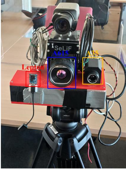
**Figure 1.** FLIR cameras used for the creation of the DASSR dataset
