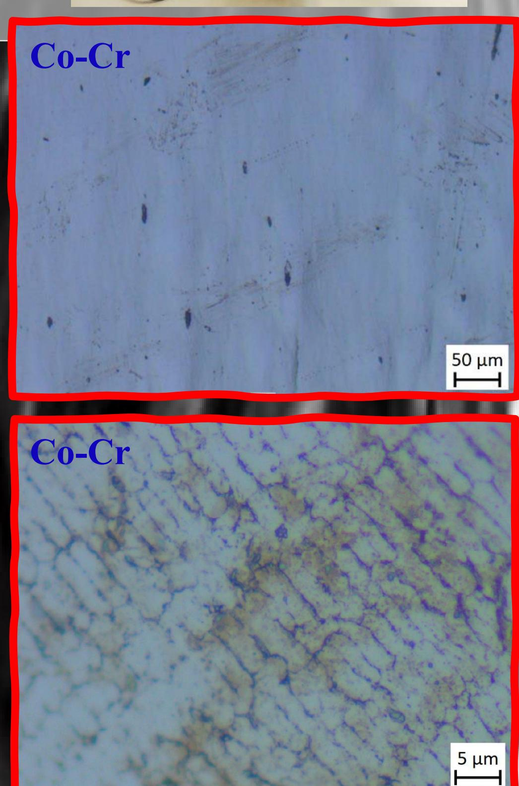
After electrochemical etching, the metallographic test is carried out by taking images with the metallographic microscope and by electrochemical test consisting in inserting a specimen into an electrochemical cell together with Saturated Calomel Electrode (SCE) as reference and Pt electrode as counter electrode. Corrosion potential (Ecorr) was determined and Electrochemical Impedance Spectroscopy (EIS) was applied.
