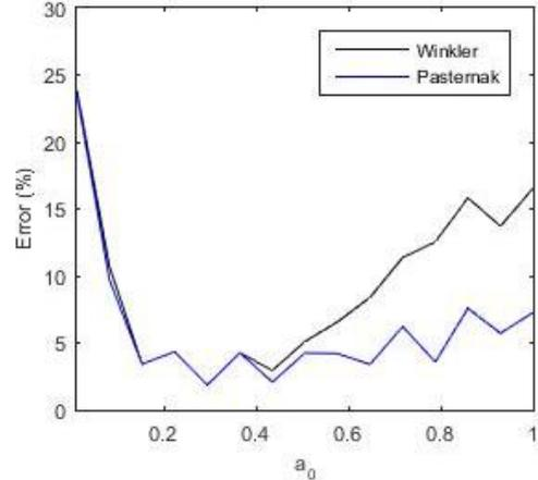
**Image 2.** Comparison of errors with respect to BEM model obtained with Winkler and Pasternak model.  $L/D = 20$ ,  $E_p/E_s = 100$ ,  $\nu_s = 0.40$ ,  $a_0 = 1$ , optimizing M
