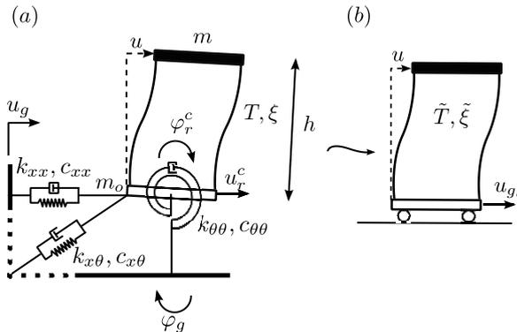
**Image 2.** (a) Substructure model of a one-storey structure and (b) equivalent single-degree-of freedom oscillator
