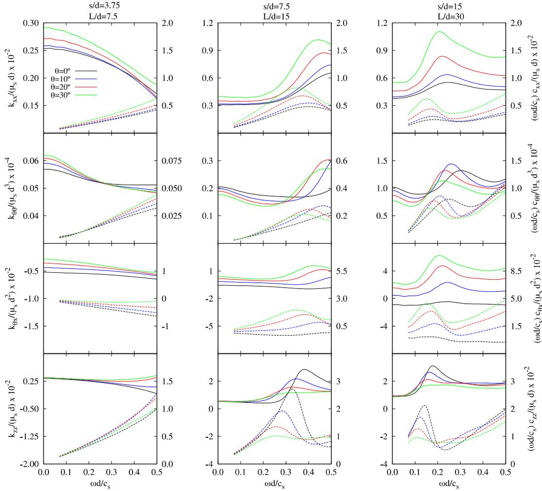
**Image 4.** Impedance functions of different  $2 \times 2$  pile groups.  $E_p/E_s = 10^3$  and  $\xi_s = 0.05$ . Solid lines to be read on left axis. Dashed lines to be read on right axis.
