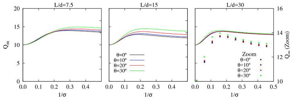
**Image 8.** Maximum structural response value for slender structures ( $h/b = 10$ ) supported on different  $2 \times 2$  pile groups with  $L/d = 7.5, 15$  and  $30$ .  $E_p/E_s = 10^3$  and  $\xi_s = 0.05$ .
