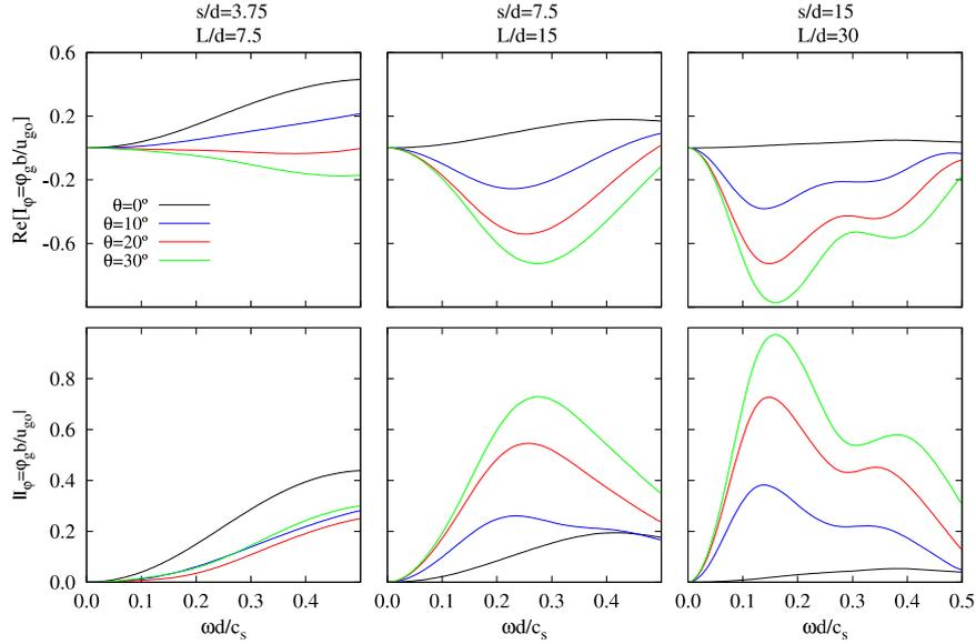
**Image 6.** Rotational kinematic interaction factors of different  $2 \times 2$  pile groups with  $L/d = 7.5, 15$  and  $30$ .  $E_p/E_s = 10^3$  and  $\xi_s = 0.05$ .
