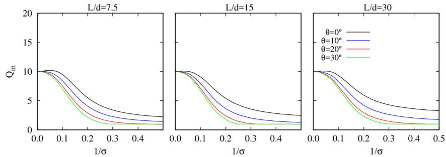
**Image 7.** Maximum structural response value for non-slender structures ( $h/b = 1$ ) supported on different  $2 \times 2$  pile groups with  $L/d = 7.5, 15$  and  $30$ .  $E_p/E_s = 10^3$  and  $\xi_s = 0.05$ .
