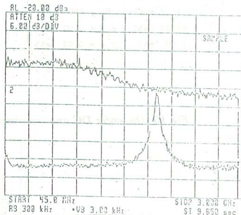
Fig.16. Optical/electrical results with an EPITAXX InGaAs PIN photodiode of 0.1 pF
