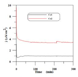
**Figure 4.** The potentiostatic polarization curves for specimens Co1 and Co2 in Ringer solution at a potential of 100 mV/ESC.
