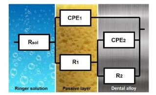
Figure 8. EC used to generate the simulated data for specimens Ni1, Ni2, Ni3, Co1, and Co2.
