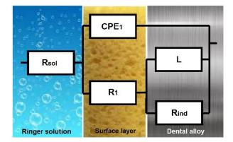
Figure 9. EC used to generate the simulated data for specimens Ni4, Ni5, and Ni6.
