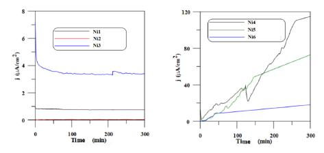
**Figure 1.** Potentiostatic polarization curves for specimens Ni1, Ni2, Ni3, Ni4, Ni5, and Ni6 in Ringer solution at a potential of 100 mV/ESC.
