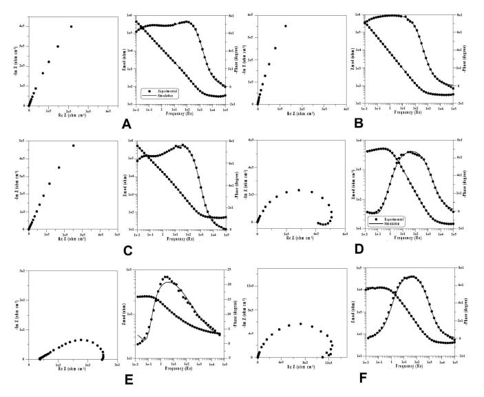
**Figure 6.** Bode spectra and Nyquist plot diagrams for NiCr-based dental alloys in Ringer solution at a potential of 100 mV/ESC. (**A**) Specimen Ni1. (**B**) Specimen Ni2. (**C**) Specimen Ni3. (**D**) Specimen Ni4. (**E**) Specimen Ni6. (**F**) Specimen Ni5.
