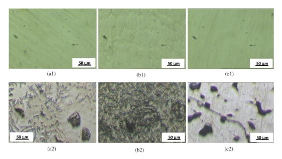
**Figure 3.** Microstructures before electrochemical treatments for (**a1**) specimen Ni5, (**b1**) specimen Ni4, (**c1**) specimen Ni6; after electrochemical treatments for (**a2**) specimen Ni5, (**b2**) specimen Ni4, and (**c2**) specimen Ni6.
