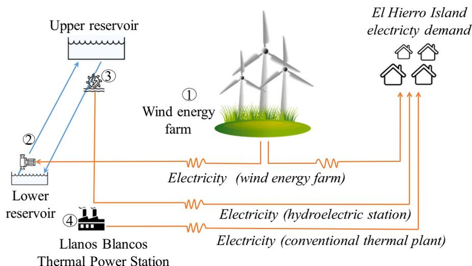
Fig. 5. Schematic representation of the Gorona del Viento wind-hydro power plant.
