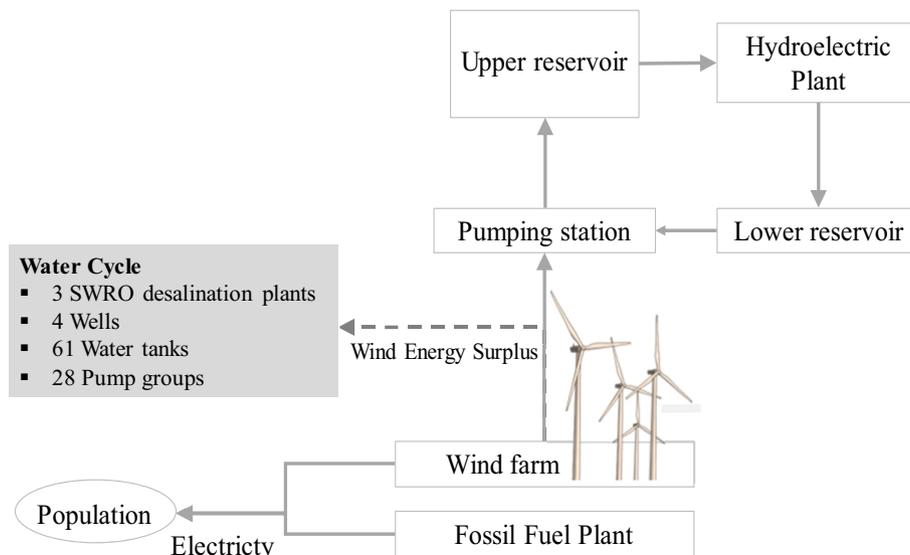
Fig. 1. Schematic diagram of the decentralised water system.
