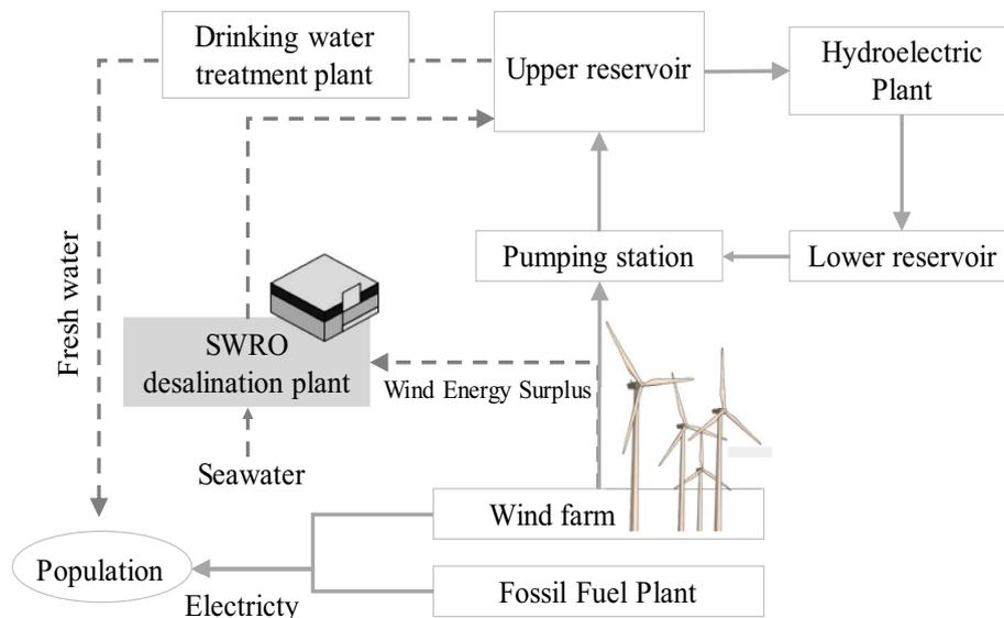
Fig. 3. Schematic diagram of the centralised water system.
