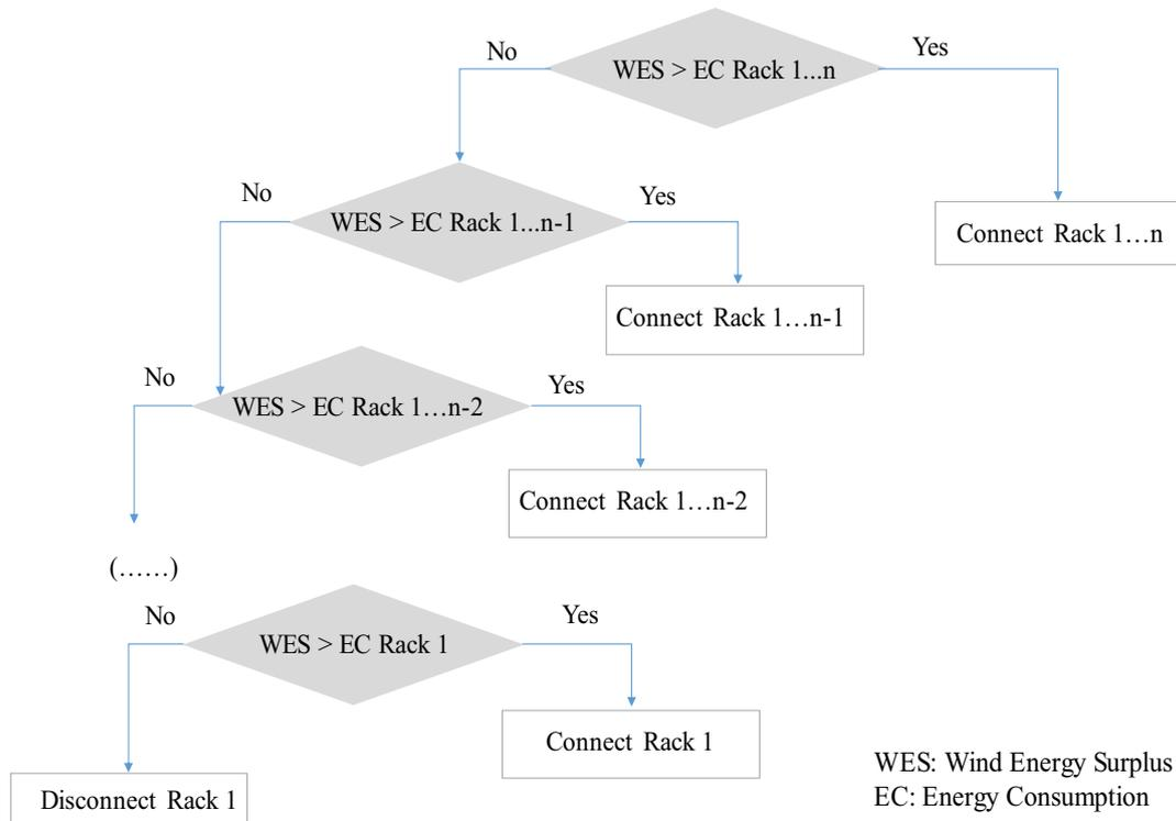
Fig. 4. Centralised water system: logic diagram of the proposed modular desalination plant operation.
