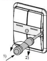
Diagram 5: Lifting out the pictogram cover
