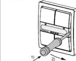
Diagram 6: Lifting out the pictogram cover
