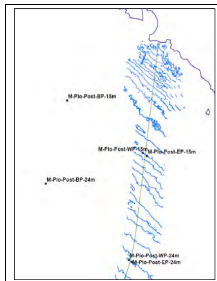
Fig.19 Location of Posidonia oceanica (sea grass) monitoring stations in the Mallorca landfall area. One station at each side (East and West) of the trench at -15 m & -24 m depth; and two Blank control stations at same depth.
