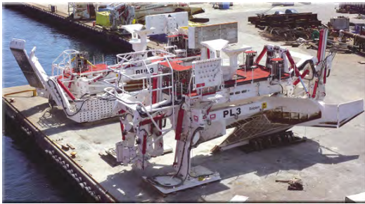
Fig.9 Image above, PL3 plough unit and behind it, a BPL3 (backfill) unit.
