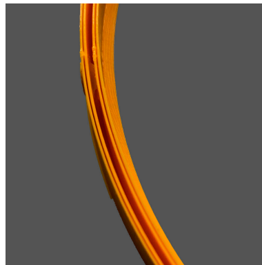
Figure 11. Walls not touching.
