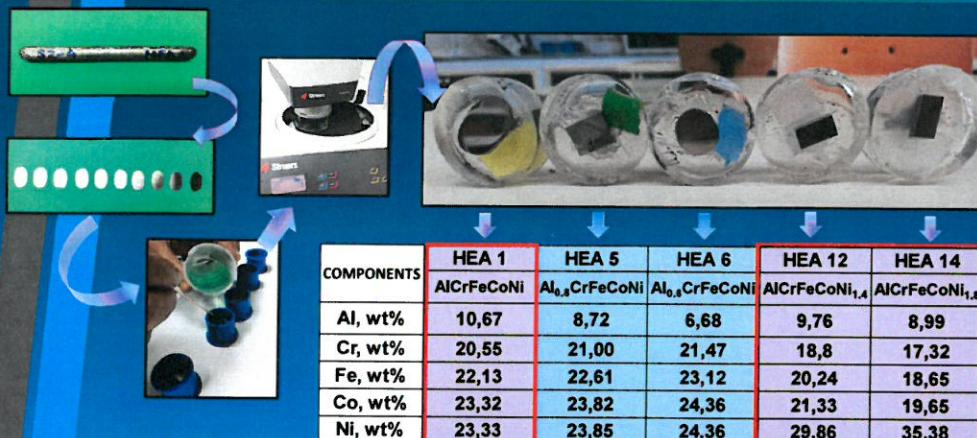
The pioneering efforts in obtaining the high entropy alloys (HEAs) created the groundwork for a new concept of solid solutions multi-principal element alloys with unique properties at the nanoscale. In this study we investigate the effect of different nickel concentration on the microstructure, hardness and corrosion properties of high entropy alloys from AlCrFeCoNi system.
