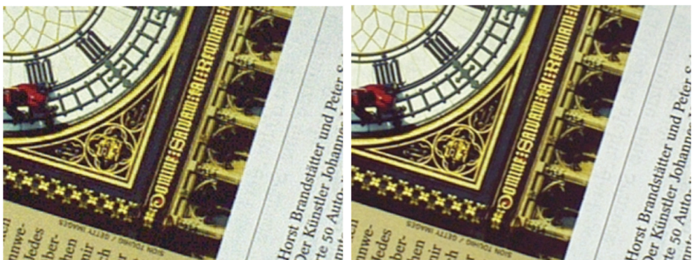
Figure 10. SmartGreen3 reconstruction with SR of "paper," frame 1 (left) and frame 20 (right). For the first frame, no SR is possible, and so it is equal to bilinear interpolation.
