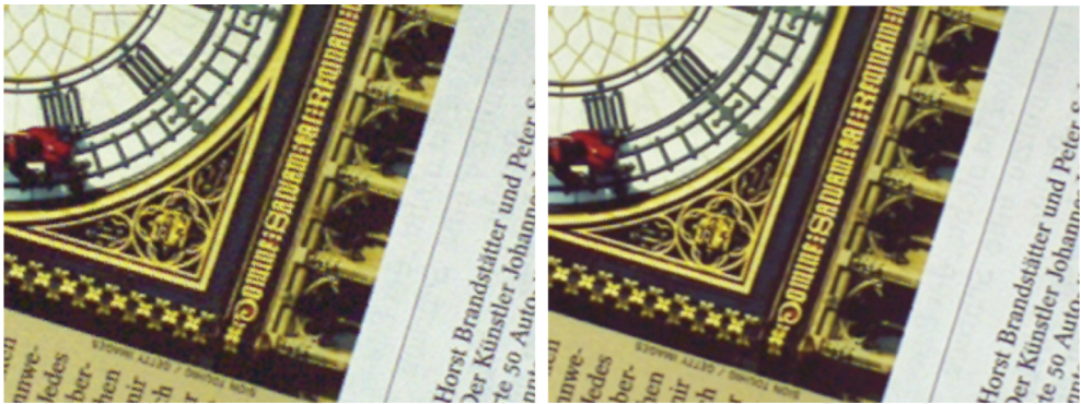
Figure 8. SmartGreen1 reconstruction with SR of “paper,” frame 1 (left) and frame 20 (right). For the first frame, no SR is possible, and so it is equal to bilinear interpolation.
