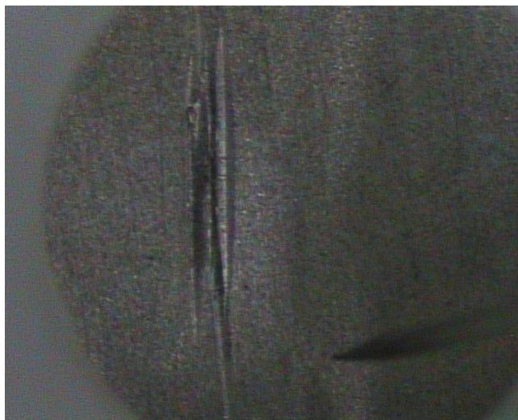
Figure 7.3.1. Optical micrograph image of a scratched zirconia-coated AA2024 sample prior to immersion in the test electrolyte. The figure also shows the SVET probe placed above the electrochemical cell containing the investigated specimen at its bottom facing upwards.
