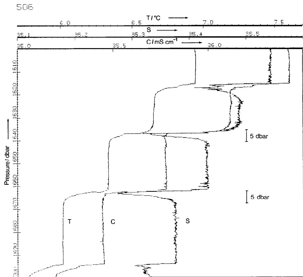
Fig. 2.2: As fig. 2.1, profiles of temperature T, conductivity C and derived salinity S between 1600 dbar and 1700 dbar.
