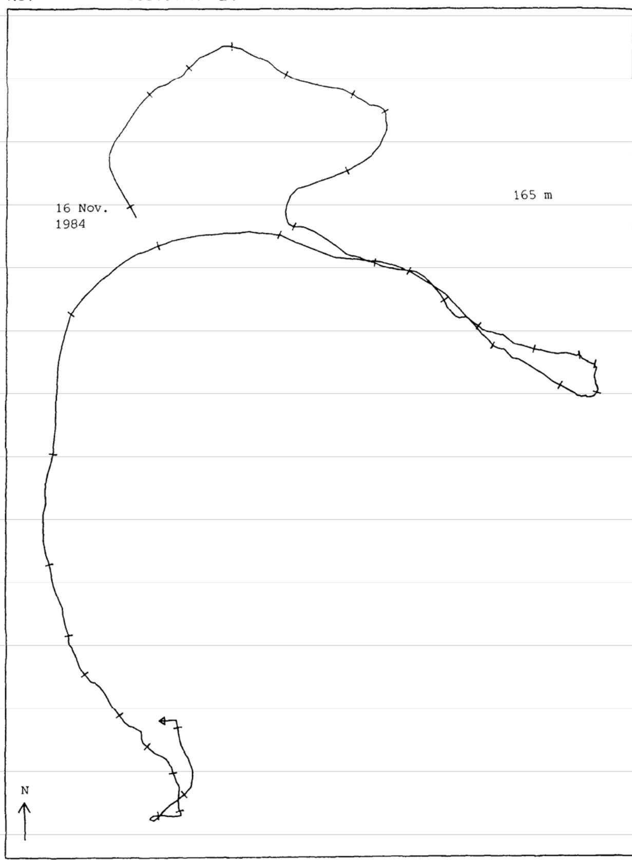
Mooring KS1/303-1: Progressive vector diagram of current in 165 m, time increments
