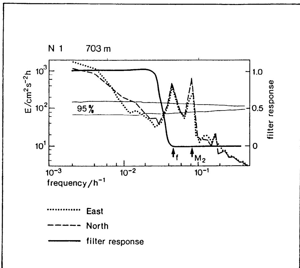
**Fig. 2.8:** High frequency spectra of current measurements at 703 m depth, position N1, 33°N, 22°W and low pass filter amplitude response according to equation 2. Adapted from Müller (1987).
