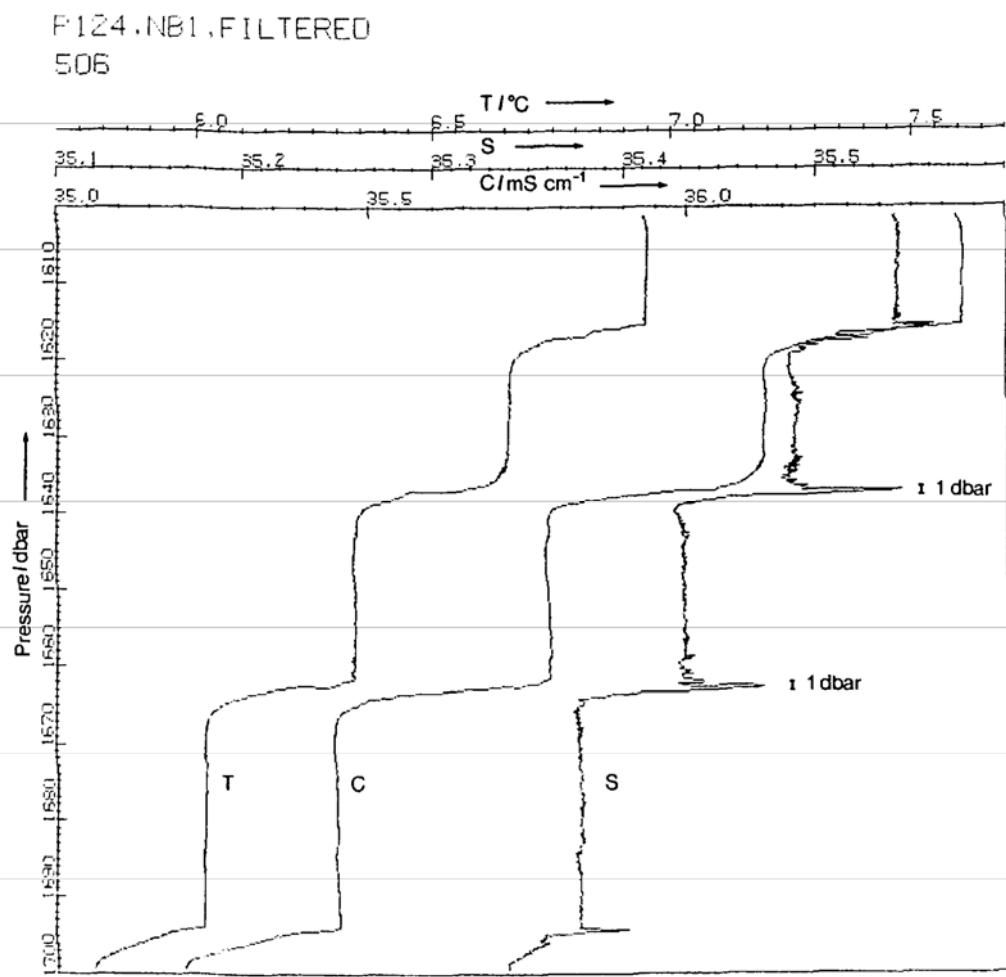
Fig. 2.3: As fig. 2.1, conductivity corrected to  $C_{i,c} = C_i + (C_{i-1,c} - C_i)e^{-\Delta t/c_k}$  with  $\Delta t/c_k = 1/9$  and S calculated anew.
