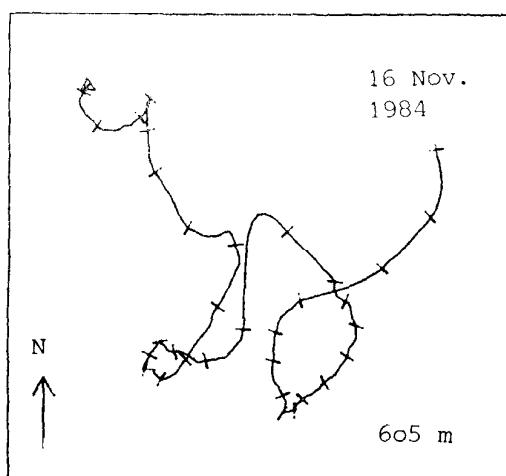
Mooring KS2/304-1: Progressive vector diagram of currents in 605 m, 1244 m and 3150 m. Time increments 10 days, start date is indicated.
