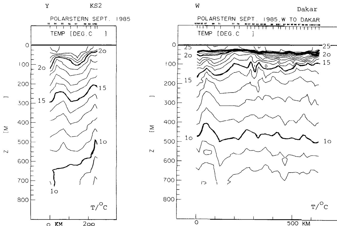
POLARSTERN cruise ANT IV/1b: XBT sections from position Y to KS2, 06-07 Oct (left) and W to Dakar, 11-13 Oct 1985 (right). See figure 1b for location of sections.
