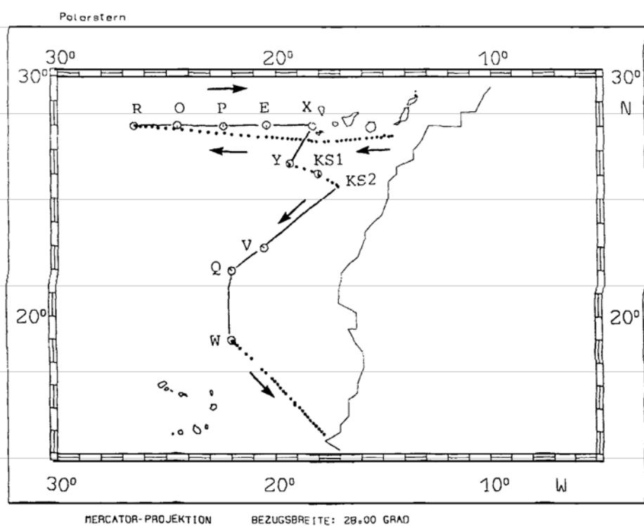
**Figure 1:** Cruise tracks of FS POSEIDON and BO TALIARTE (a) and FS POLARSTERN (b) in autumn 1985 with CTD-stations (circles), bottle stations (triangles), and XBT casts (points). Mooring positions are denoted with letters.
