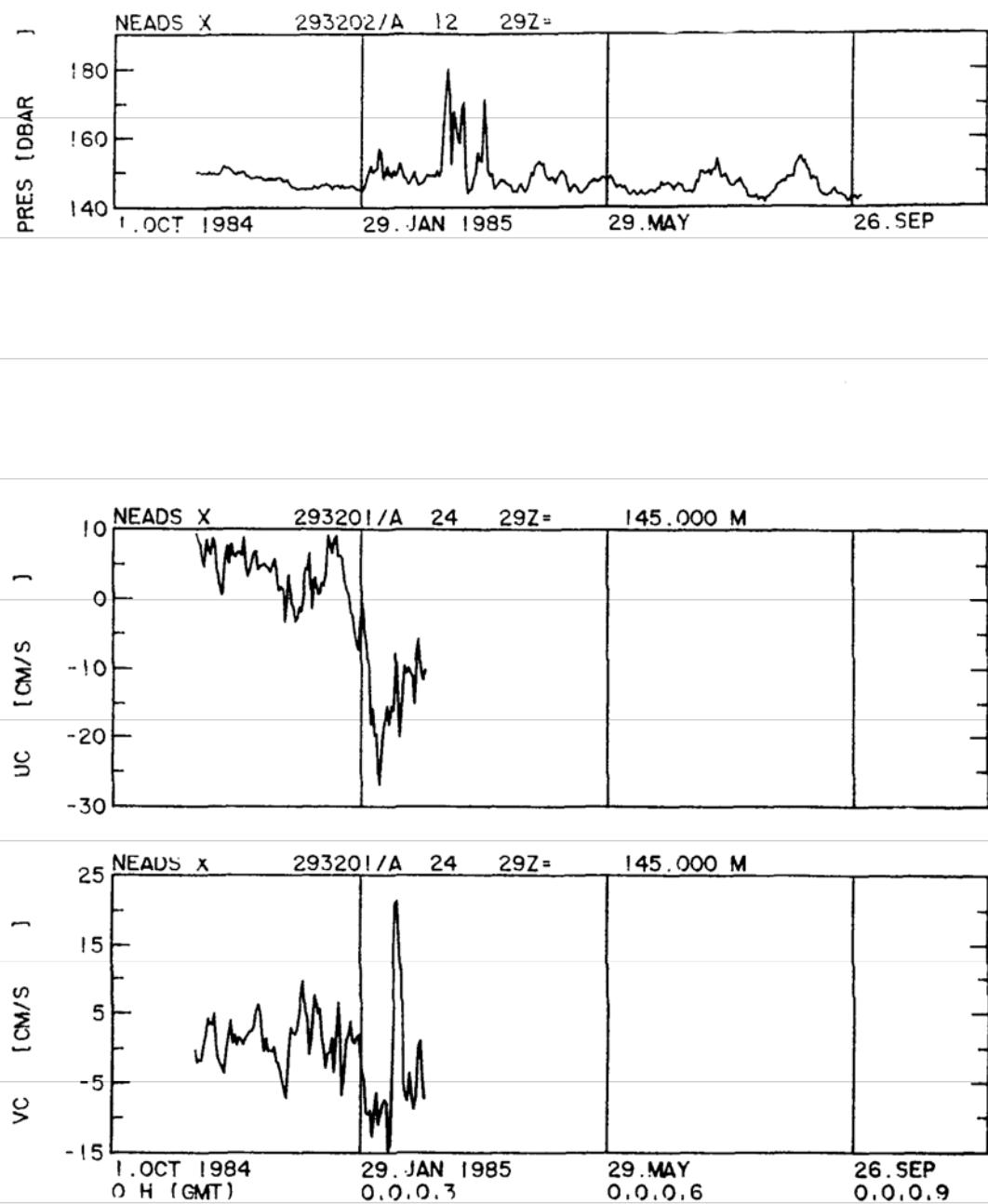
Mooring X/293-2: Time series of pressure (upper figure), east component (uc) and north component (vc) of current in 145 m.
