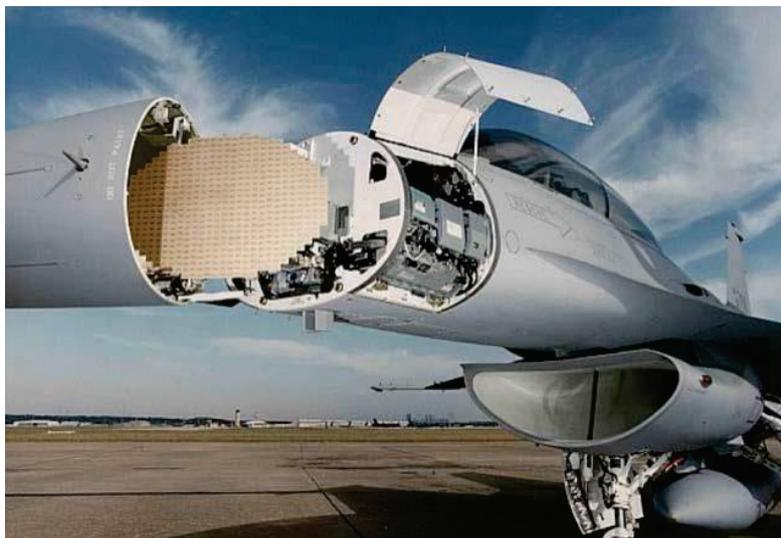
Figura 1. Antena *phased array* [1].
