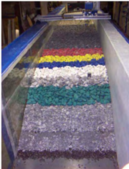
Fig. 4: Large wave-flume (1/40), front view of Shield Reef Breakwater
