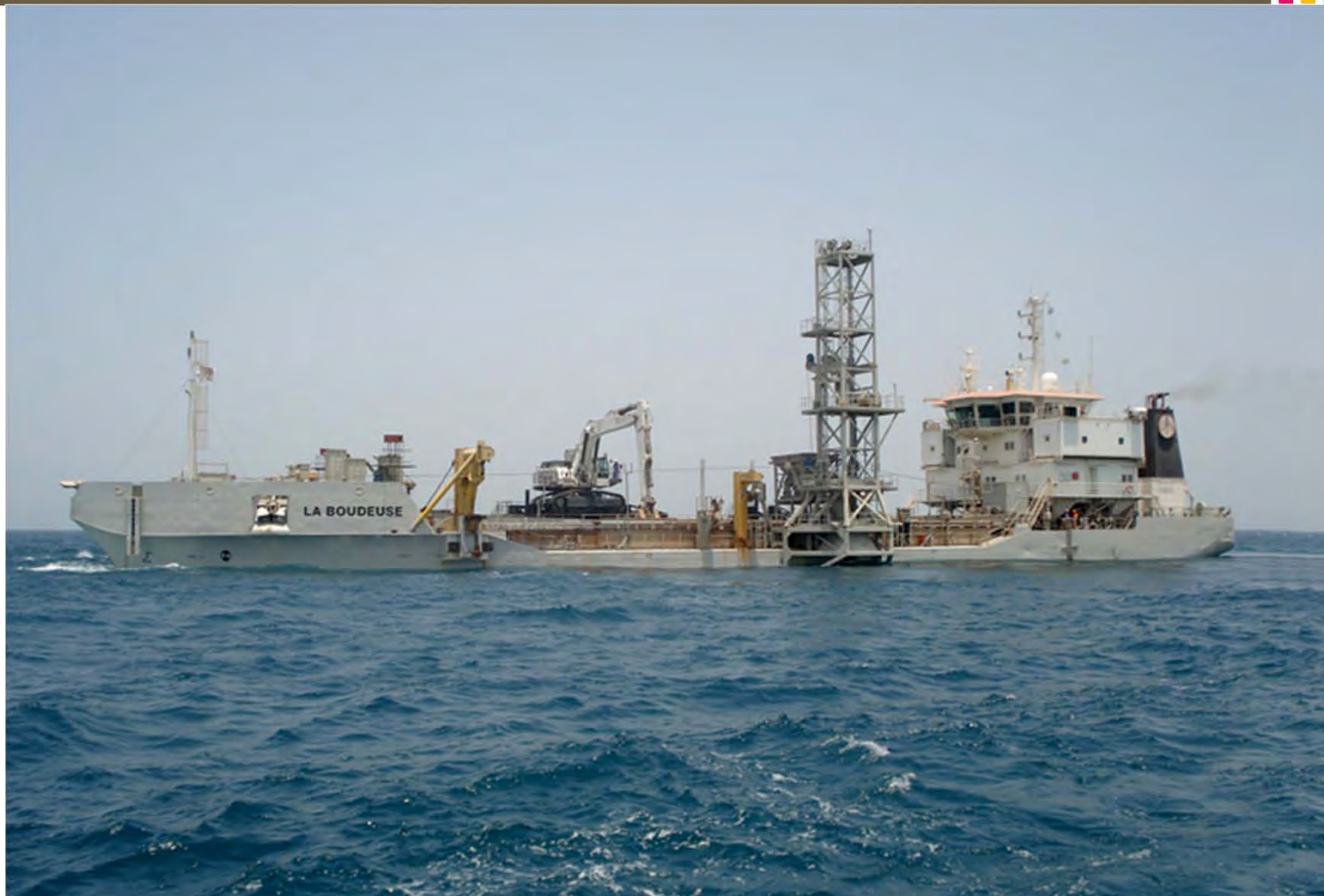
La Boudeuse | Dynamic Positioned Flexible Fall Pipe Vessel
