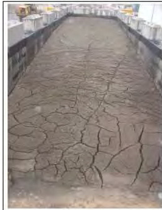
Day 36: Crust-drying with superficial cracks
