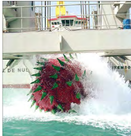
The CSD “JFJ De Nul” cutter dredger with worldst largest cutter-power
