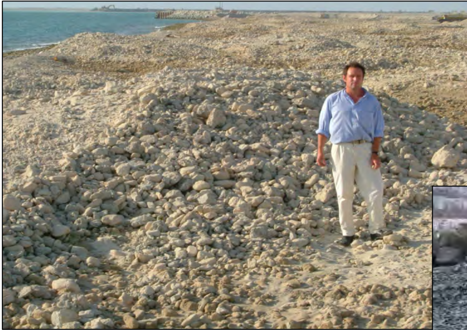
Cap-Rock dredged by CSD (Persian Gulf)
