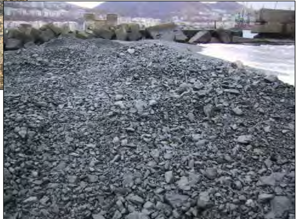
Tertiary Claystones dredged by CSD "JFJ DE Nul" (UCS = 11 MPa)
