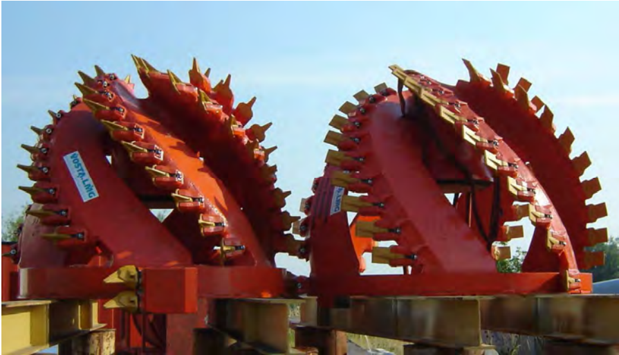
Cutterheads fitted with Pickpoints (left) or Cutter-Teeth (right)
